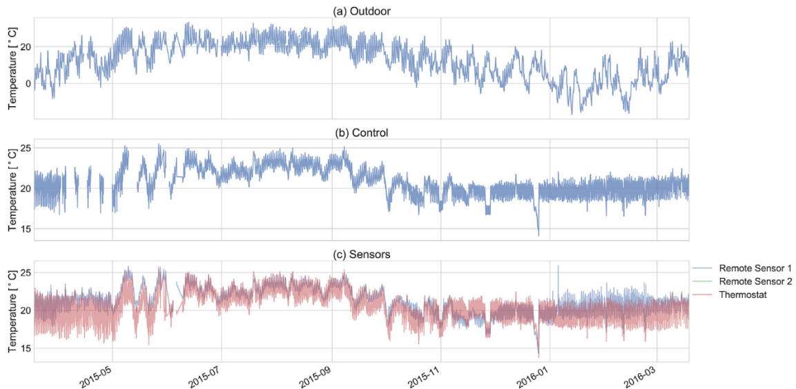
Fig. 5. Sample of the (a) outdoor temperature data, (b) control temperatures, and (c) sensor temperatures for a single thermostat found in the ‘Donate Your Data’ dataset.
